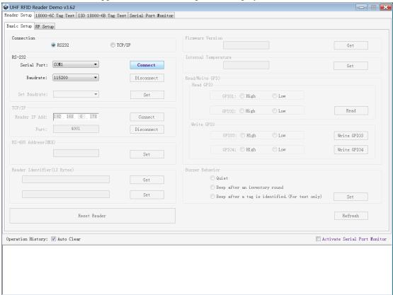
Please select RS232 in Connection if the reader is connected via RS -232 port. Selecting the corresponding Serial Port number and Baudrate, default baudrate is 115200. As illustrated below:
