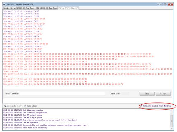
Note: Response speed of Demo will be slow down after opening the **Activate Serial Port Monitor**. Generally, this function should be turn off.
