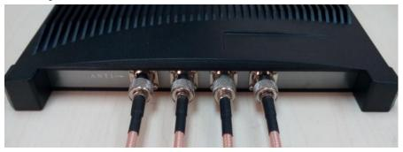
Note: The antenna(s) port to reader is TNC male port, and the gain of antenna(s) is less than 6dBi.
