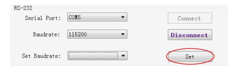
After setting successfully, new baud rate will be saved in the FLASH inside of reader and won't lose after power cut. But the baud rate communicate with the reader must be new.
