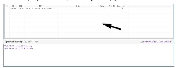
How many tags operated successfully, the equal of pieces data will be displayed in **Tag List**. It is blank in **Data** and this is the difference from **Read Tag**. The user can read the tag again in the same area to verify if the data was written correctly.
