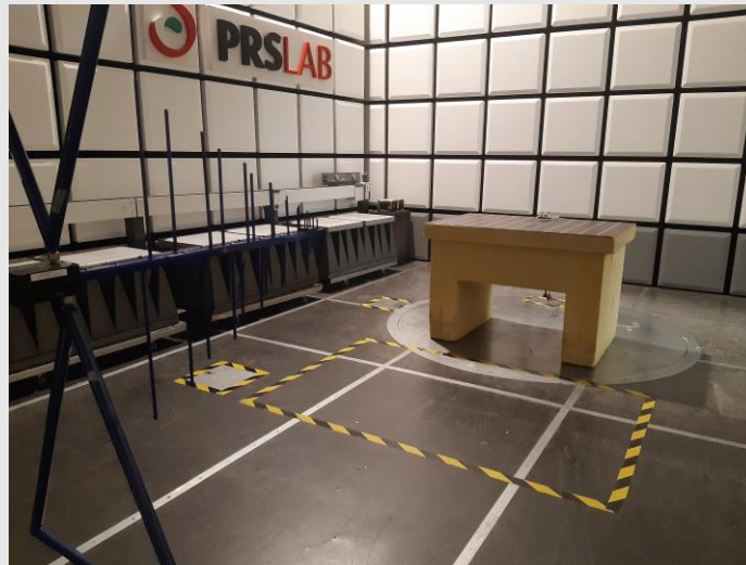
PHOTO N° 3 – SETUP FOR RADIATED EMISSIONS 30MHz – 1GHz
