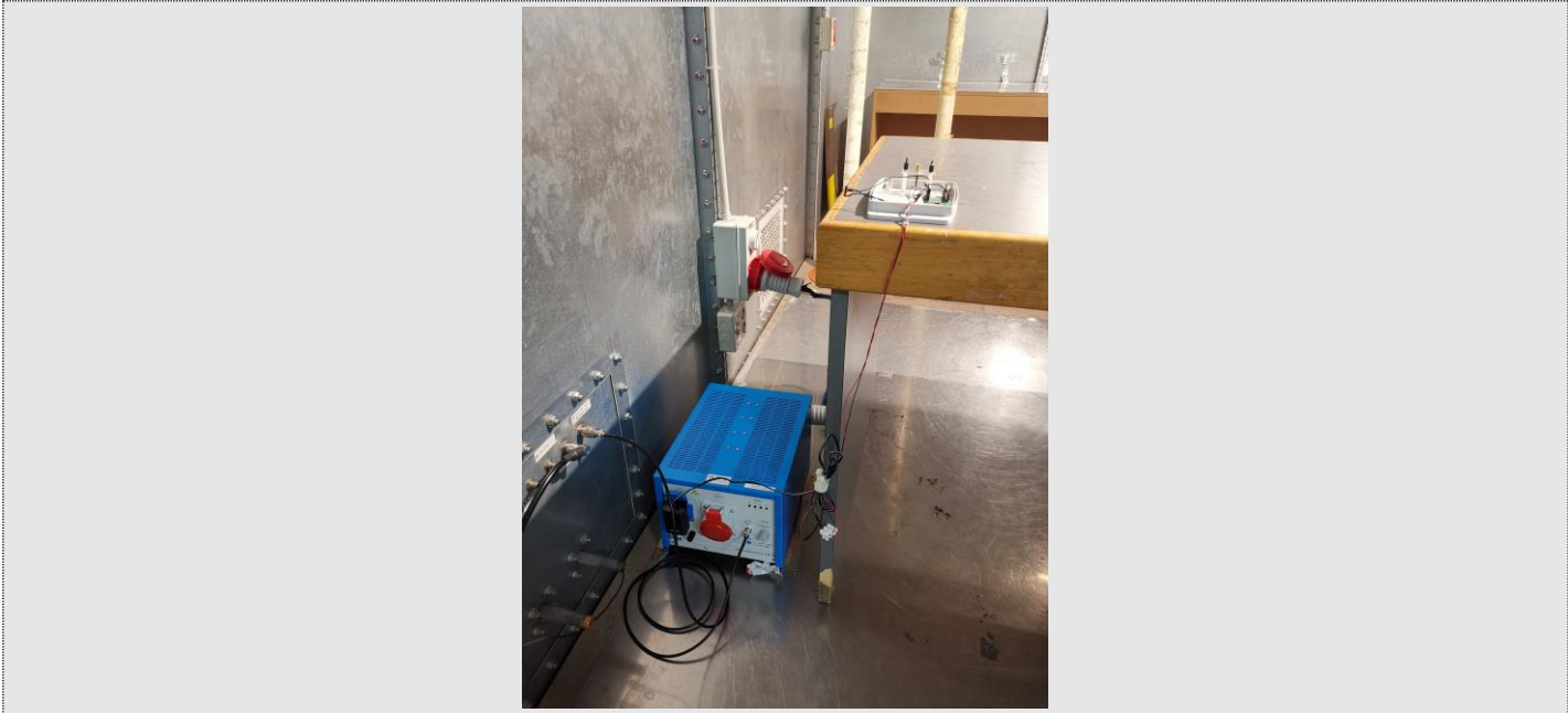
PHOTO N° 4 – SETUP FOR CONDUCTED EMISSIONS 150kHz – 30MHz
