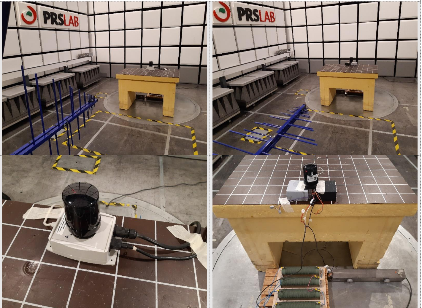
PHOTO N° 2 - RADIATED EMISSION TEST SETUP
