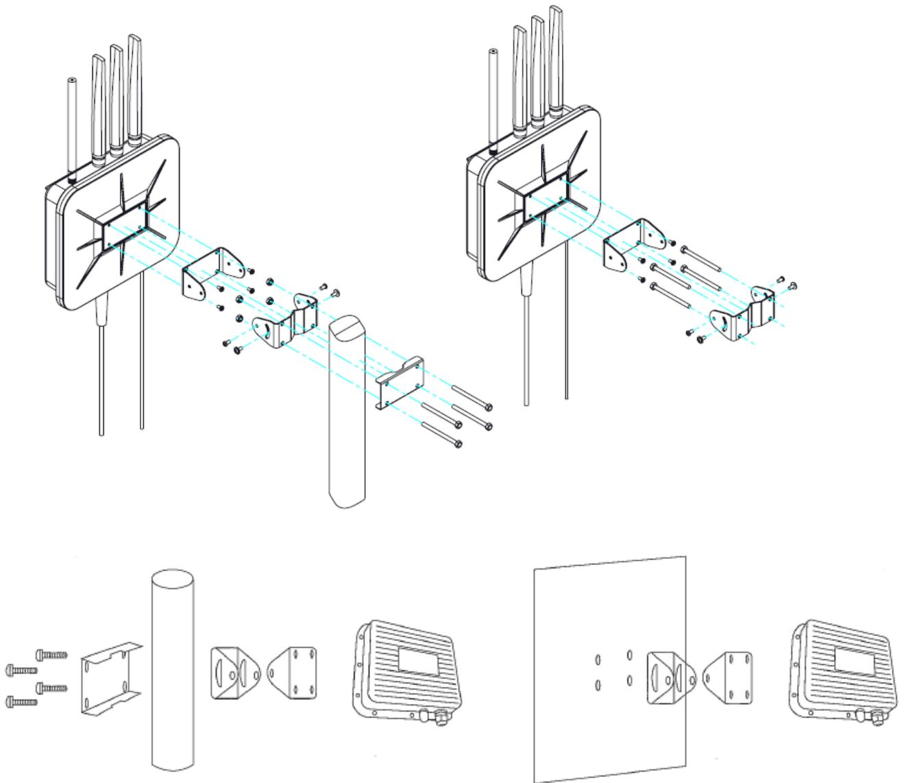
**Figure 2** Instructions for mounting PE.AMI Gateway on a pole (left side) and on a flat surface (right side).
