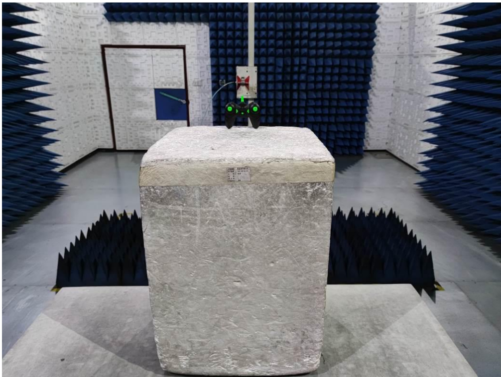
RADIATED EMISSION TEST SETUP ABOVE 1GHz
