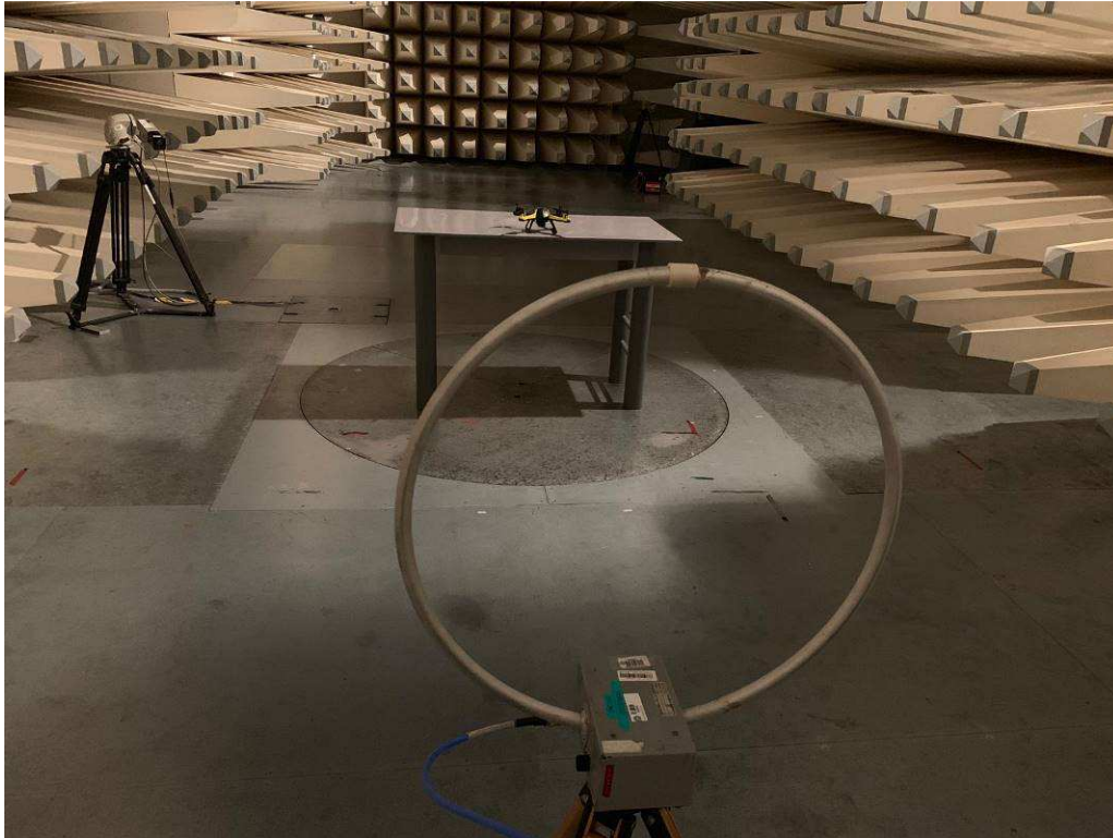
Setup for Radiated Emission
