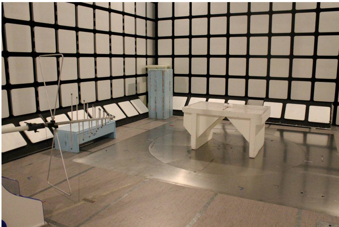
Photograph 2. Radiated Spurious Emissions 30 – 1000 MHz
