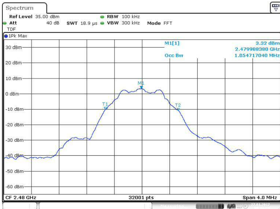
Figure 19: 99% OBW channel high
