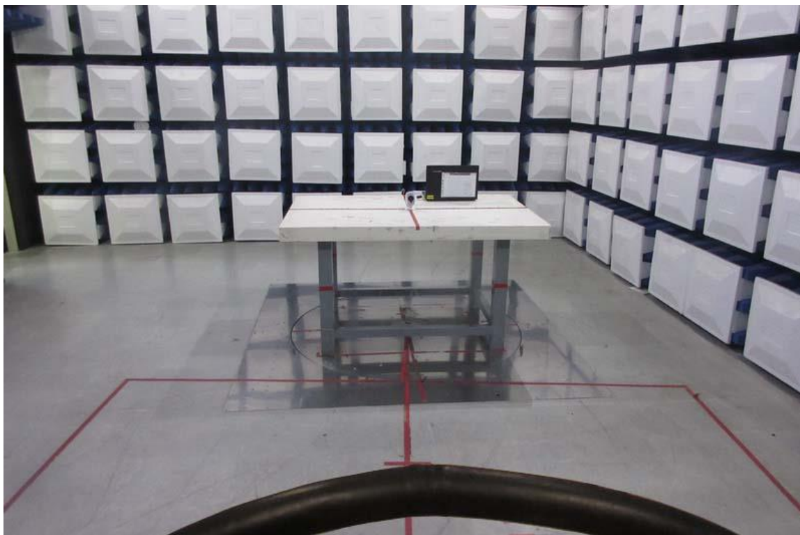
Photograph 2: Set-up for Spurious Emissions (30MHz-1GHz)
