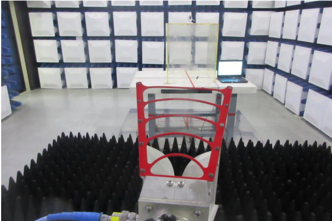
Photograph 4: Set-up for Spurious Emissions (18GHz-26GHz)
