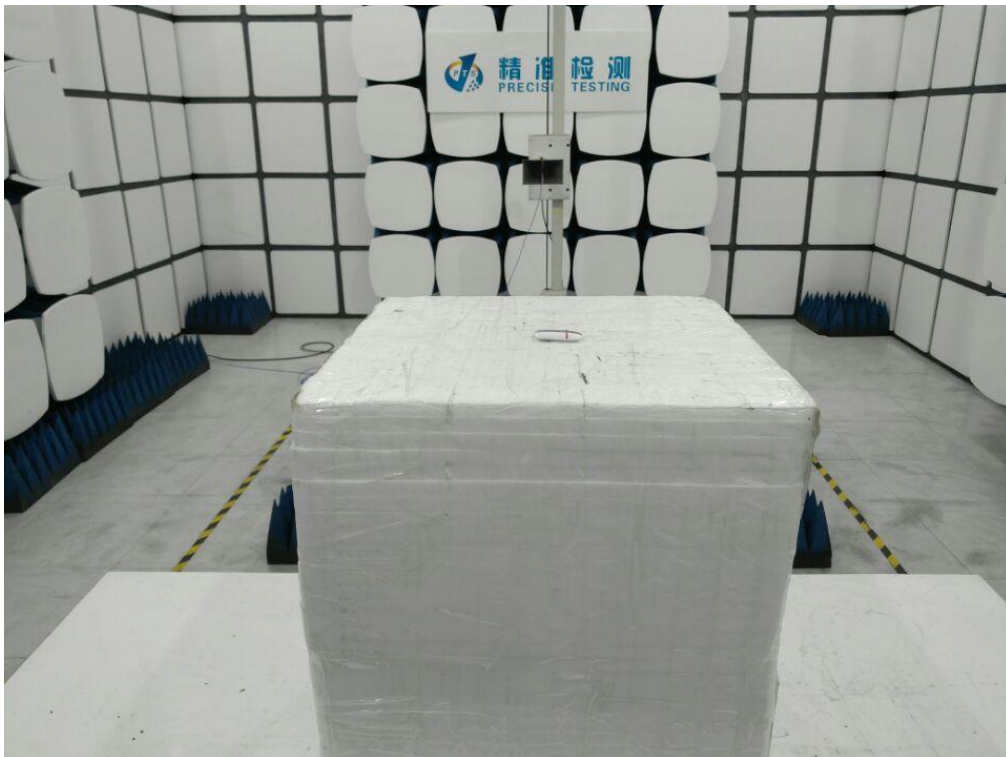
RADIATED EMISSION TEST SETUP ABOVE 1GHz
