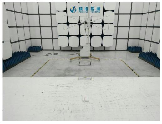
RADIATED EMISSION TEST SETUP ABOVE 1GHz
