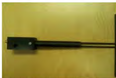
Figure 1 – MVG COMOSAR Validation Dipole
