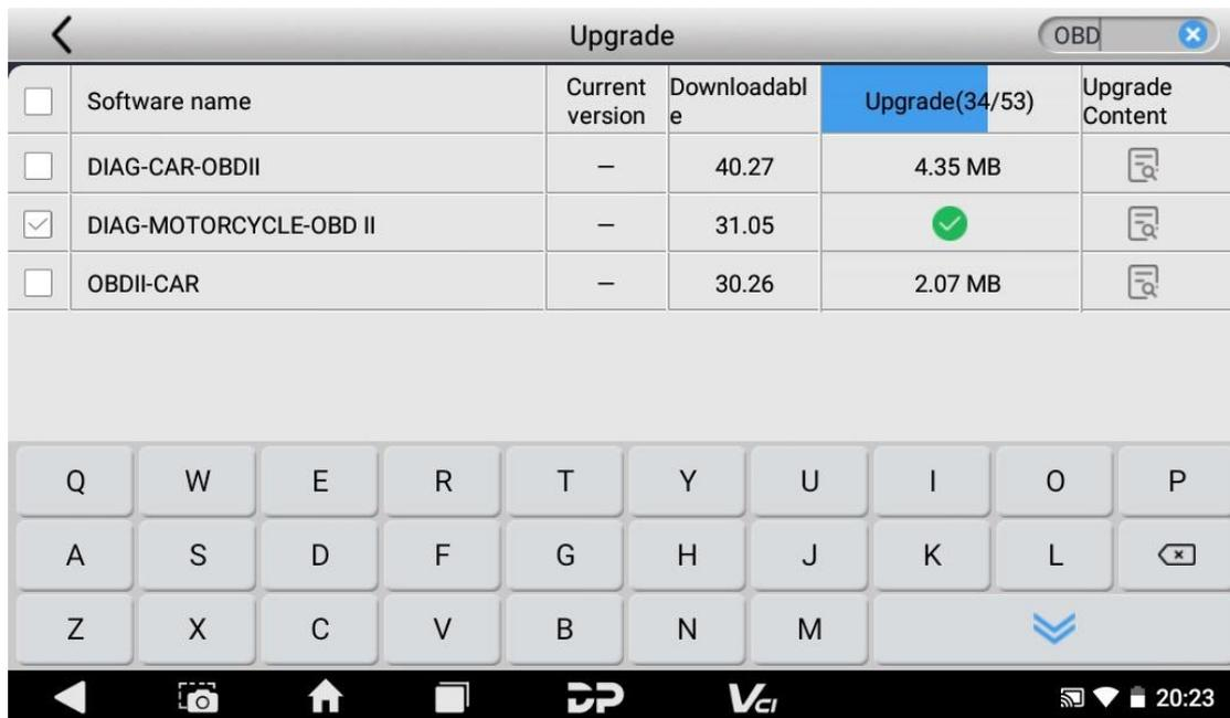
After the upgrade is completed, you can enter the diagnostic programming to view the upgrade version description and the version number, and you can perform related diagnostic operations and functions.
