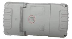
In the case of power on, long press the printer test key for three seconds, the printer will automatically print a section of self-test content, indicating that the printer function is normal. FCC Statement:
