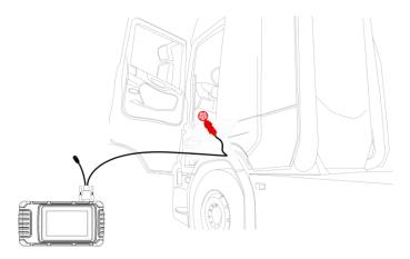
Note: at this time, the equipment is powered by the vehicle diagnostic port, and the device starts up automatically. If
