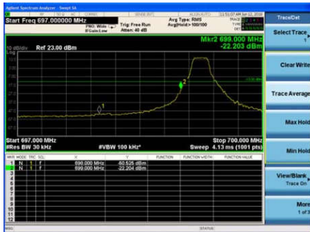
LTE Band 12 16QAM 5MHz CH-Low, 1 RB
