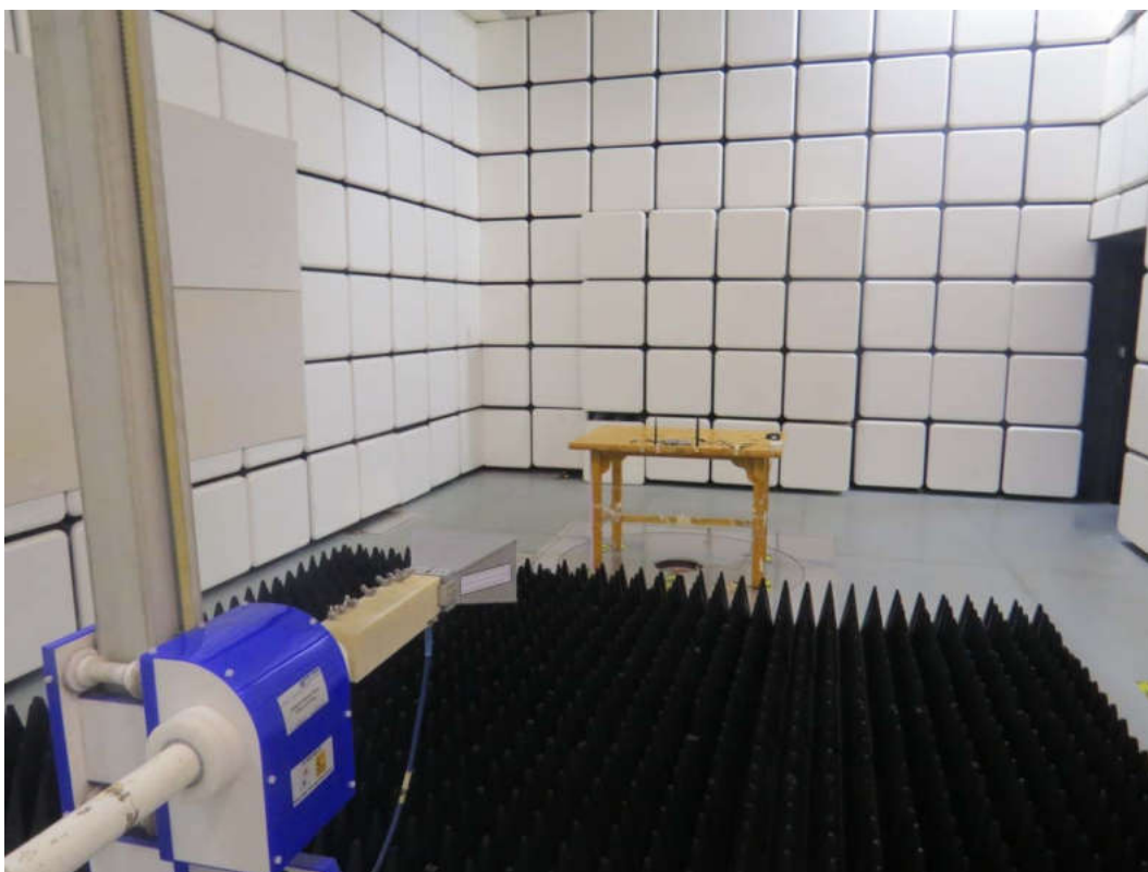
Picture 2: Radiated Spurious Emissions Test setup
