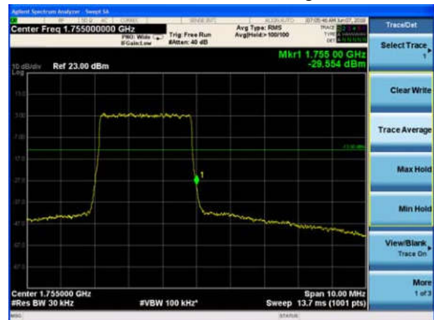
LTE Band 4 QPSK 5MHz CH-High, 1 RB
