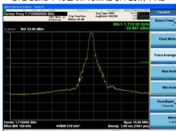
LTE Band 4 16QAM 20MHz CH-Low, 1 RB
