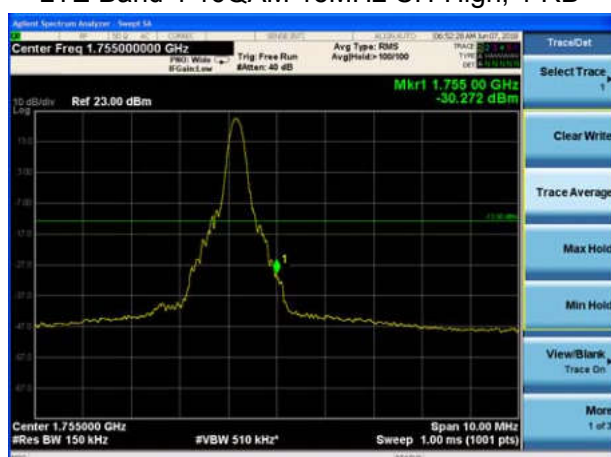
LTE Band 4 16QAM 20MHz CH-High, 1 RB
