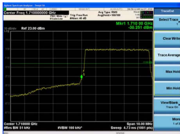
LTE Band 4 QPSK 5MHz CH-Low, 100%RB
