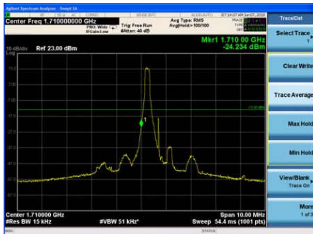
LTE Band 4 QPSK 1.4MHz CH-Low, 100%RB
