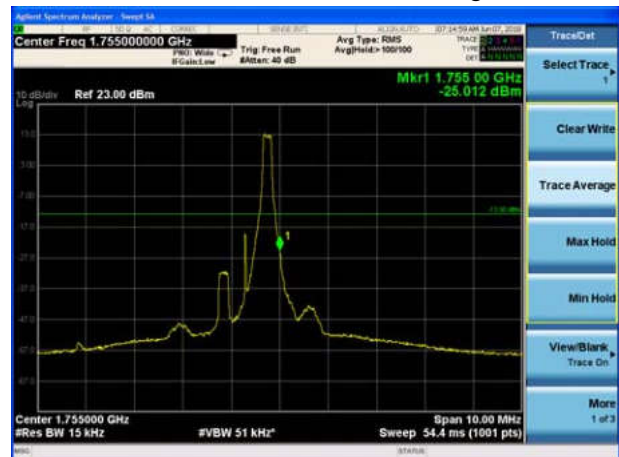
LTE Band 4 QPSK 1.4MHz CH-High, 100%RB
