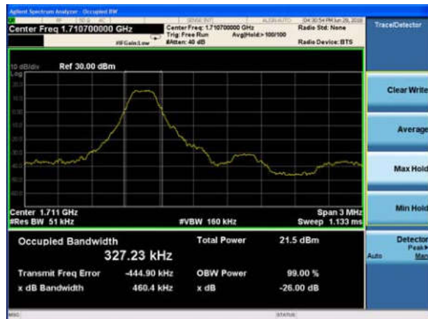
LTE Band 4 16QAM 1.4MHz CH-Middle
