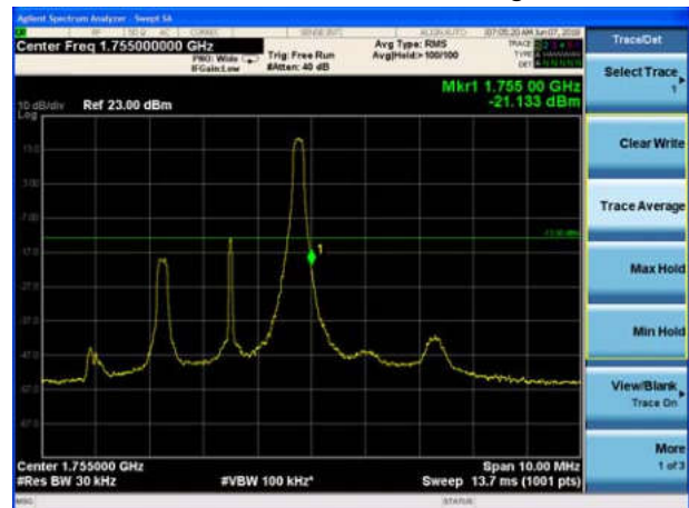
LTE Band 4 QPSK 3MHz CH-High, 1 RB
