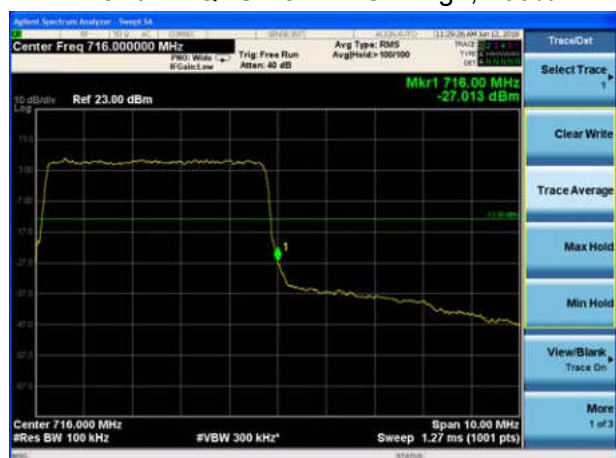
LTE Band 12 QPSK 10MHz CH-High, 1 RB
