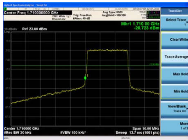
LTE Band 4 QPSK 5MHz CH-Low, 1 RB
