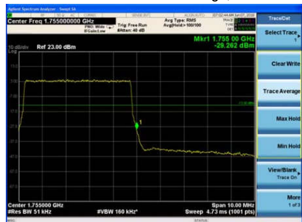
LTE Band 4 QPSK 5MHz CH-High, 100%RB
