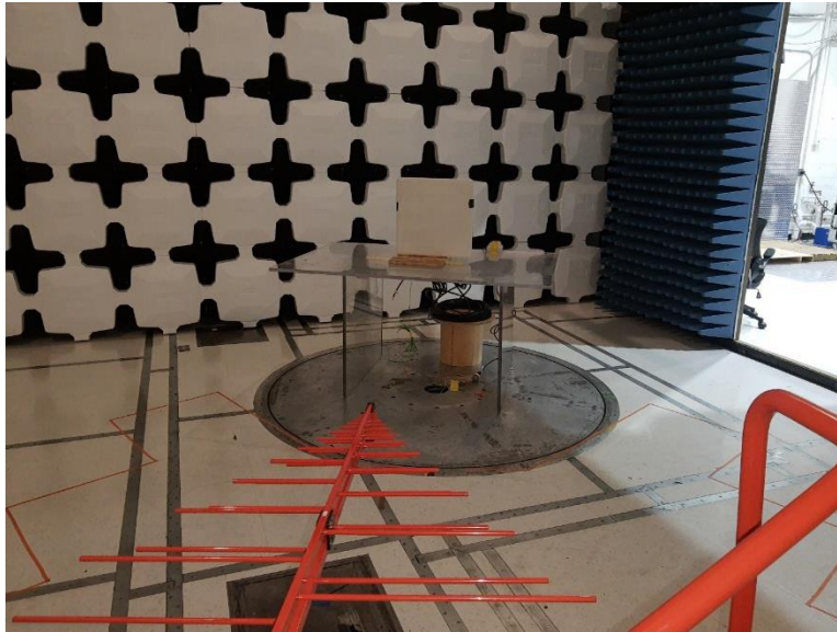
Figure 175. Radiated Emissions Test Setup below 1GHz - 13dBi Antenna
