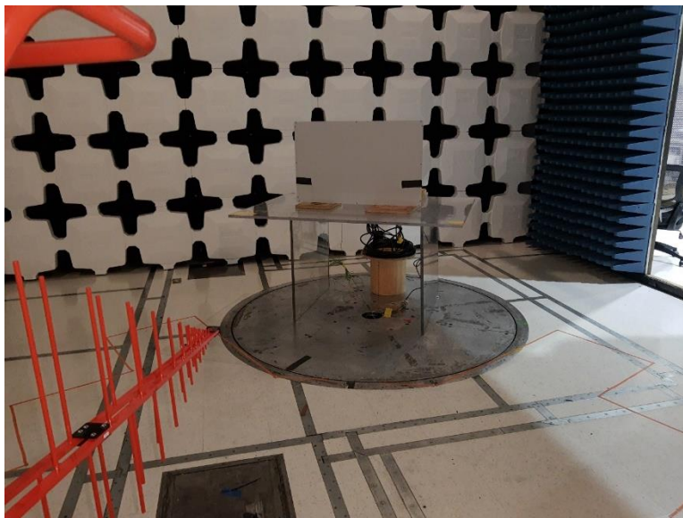
Figure 176. Radiated Emissions Test Setup below 1GHz - 15dBi Antenna
