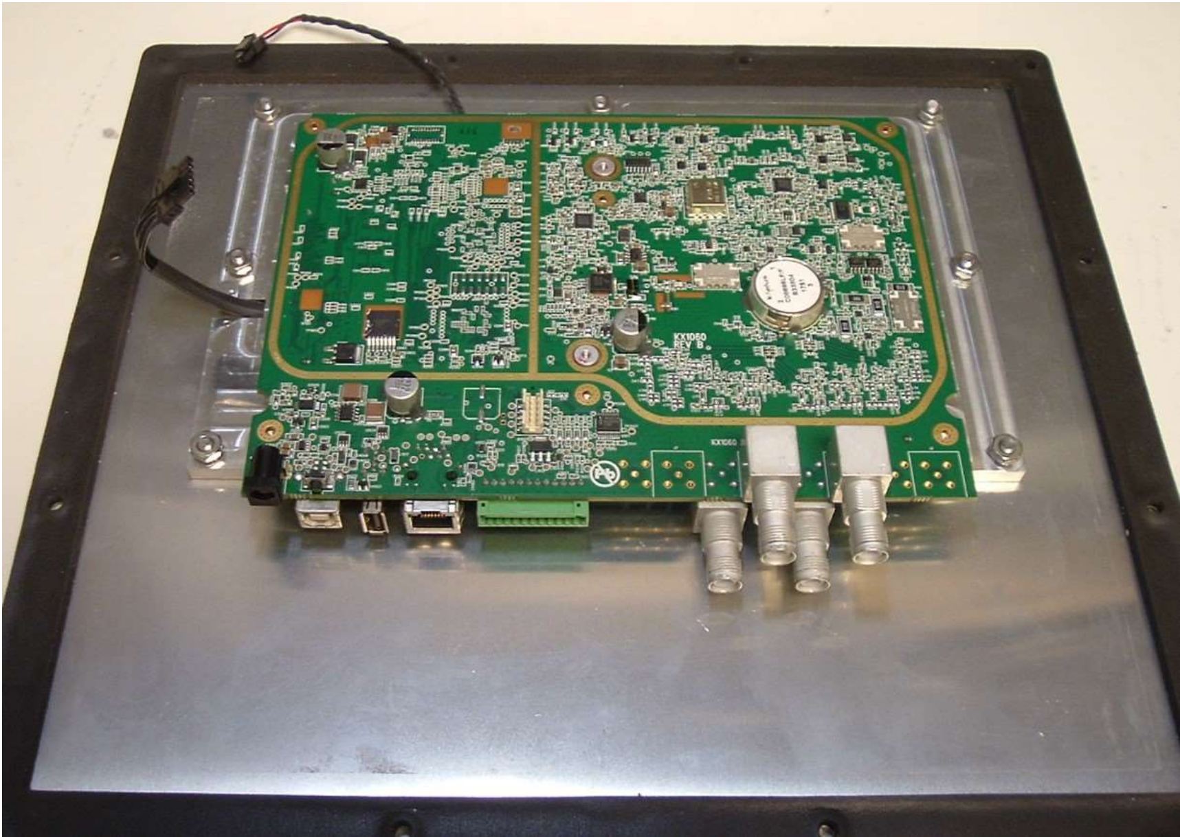
Internal Photo #7: 6204 PCB Assembly Bottom (Bottom Shield Cover Removed, PCBA Still Mounted)
