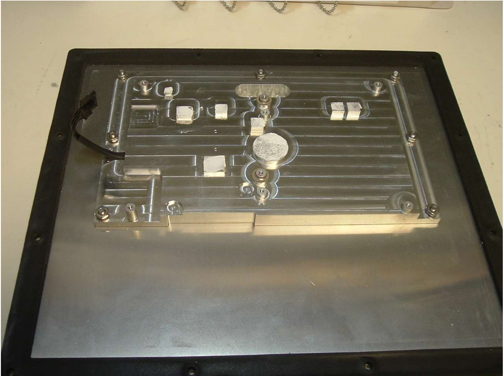
Internal Photo #13: 6204 Assembly Base Plate Mounted to Interior Surface of Enclosure Lid
