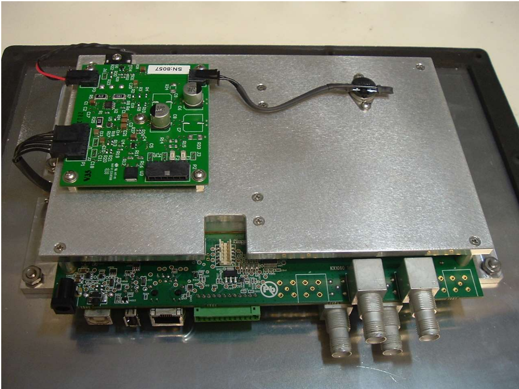
Internal Photo #5: 6204 Bottom Shield Cover, Daughter PCB Assembly & Interconnect Wiring (Close-Up View)
