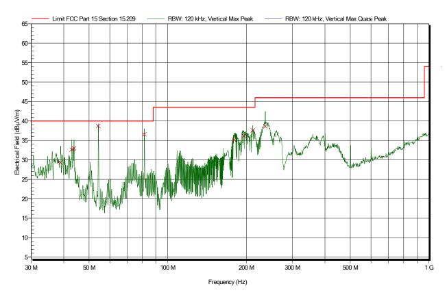
Higher signals, maximized and re-measured with quasi-peak detector
