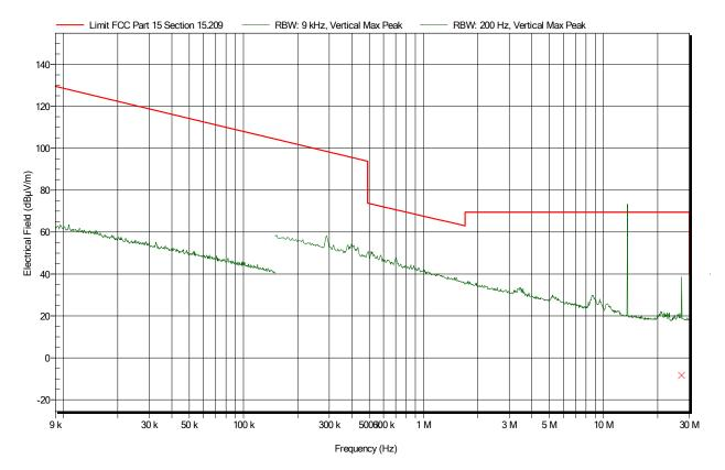
Higher signals, maximized and re-measured with quasi-peak detector
