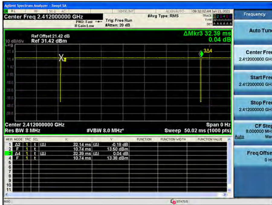
Duty cycle plot (802.11b(1 Mbps))
