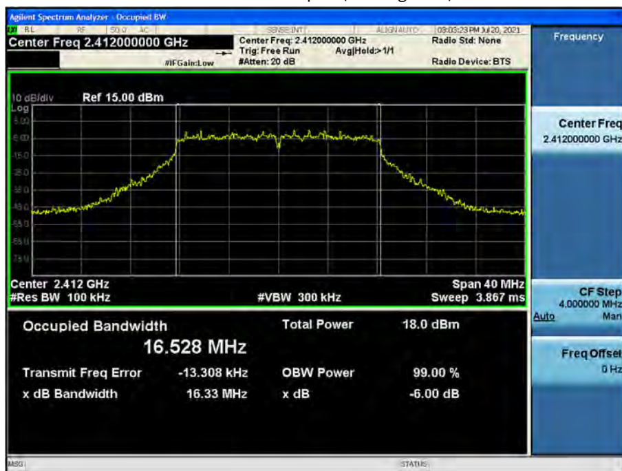
6 dB Bandwidth plot (802.11g-CH 1)
