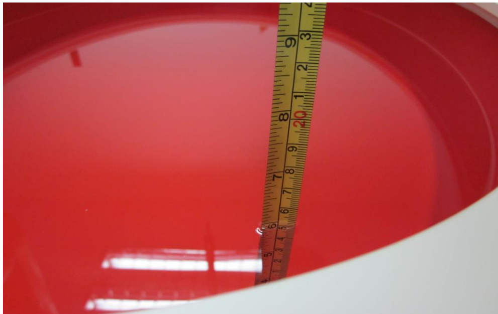
Figure 4.4: Liquid depth in the Flat Phantom
