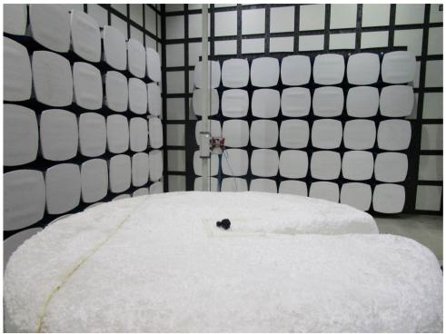
1.2 Radiated Spurious Emissions Test Setup
