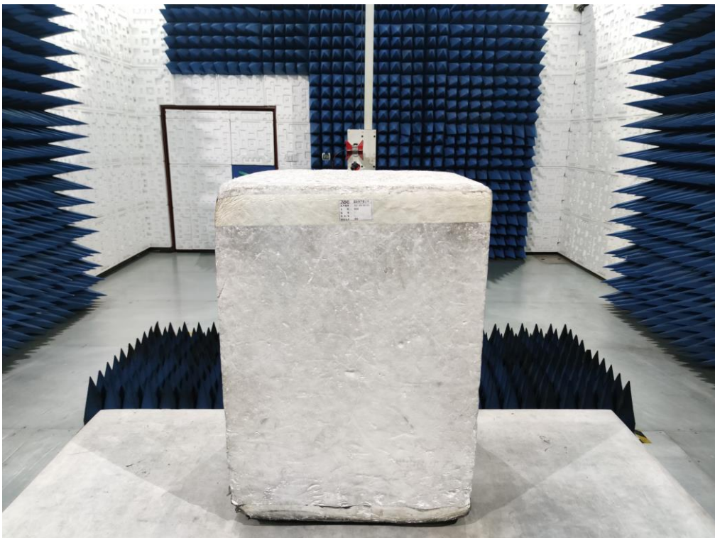
RADIATED SPURIOUS EMISSION ABOVE 1G TEST SETUP
