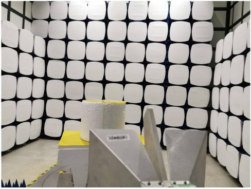
1.2 Radiated Spurious Emissions Test Setup
