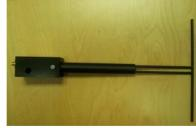
Figure 1 – MVG COMOSAR Validation Dipole
