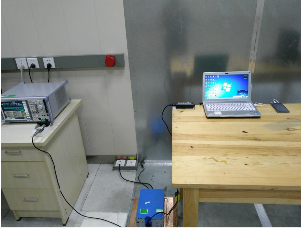
FCC RADIATED EMISSION TEST SETUP
