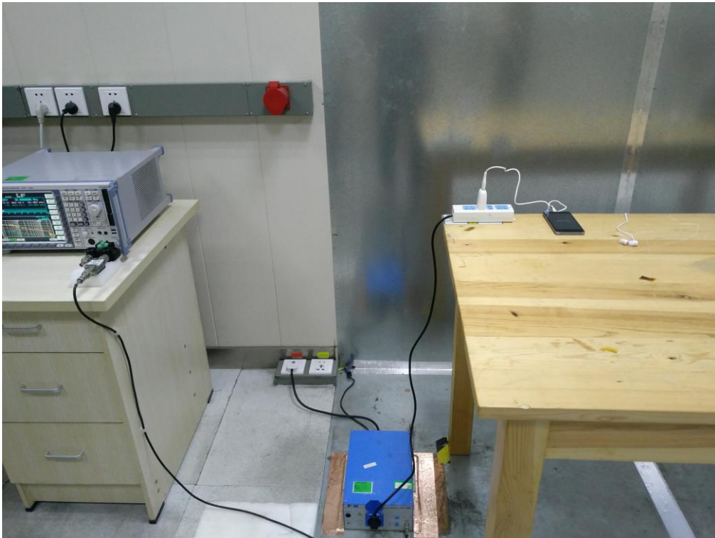
FCC RADIATED EMISSION TEST SETUP
