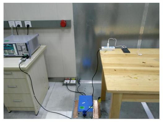
FCC RADIATED EMISSION TEST SETUP
