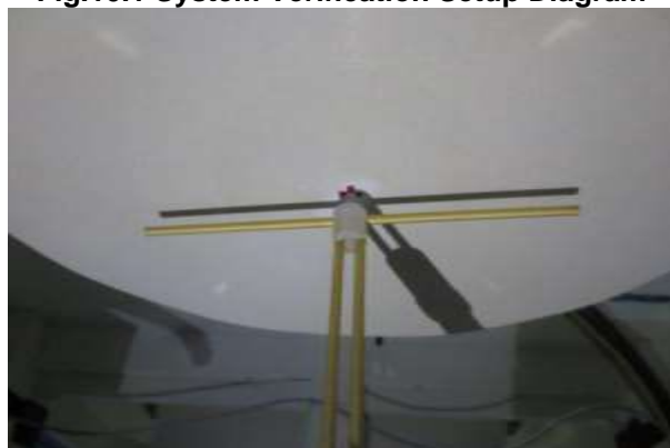
Fig.10.2 Photo of Dipole setup
