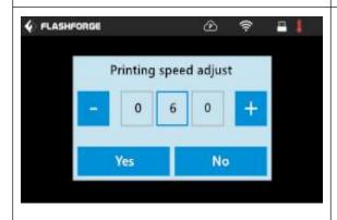
To set the printing speed during printing: Tap [Yes] to save the setting while tap [No] to cancel the setting.
