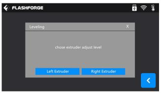
(5-2) Tap to choose extruder adjust level: Use Left or Right extruder to do the leveling.
