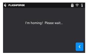
(5-1) Tap [Level] to start leveling. Wait while the extruder and platform finish homing movements.
