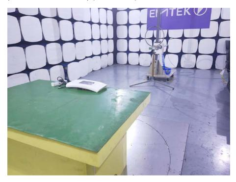
Spurious Emission Test Setup (30MHz-1GHz)
