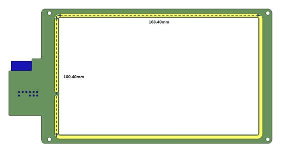
For RS128, the NFC antenna is a single loop antenna routed on a 2-layer pcb as shown above. The dimension is 168.4mm x 100.4mm with trace width of 3mm.
