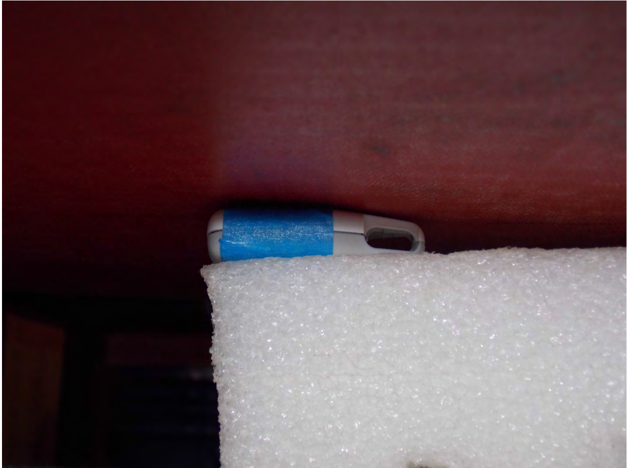
Test Position Back 0 mm Gap
