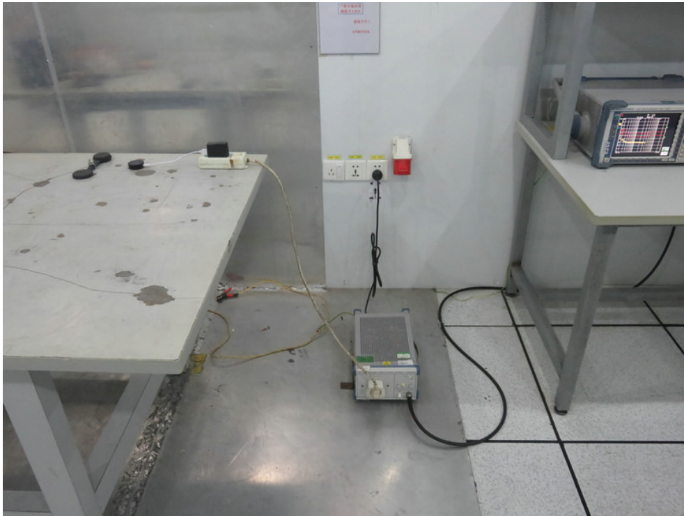
Photo of Conducted Emission Measurement
