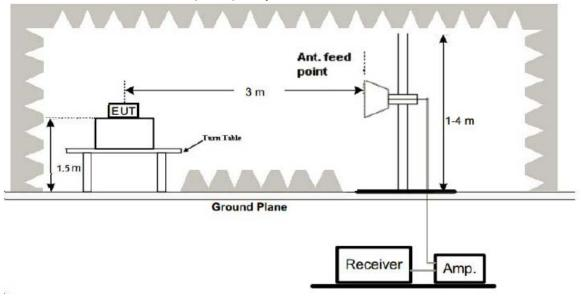
(3) Radiated Emission Test-Up Frequency Above 1GHz
