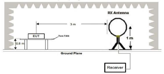
(2) Radiated Emission Test-Up Frequency 30MHz~1GHz
