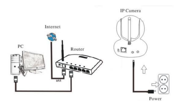
Connect the Camera with Internet cable and power accordingly as above
