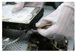
Step 3: Connect the power cable to the HDD.
