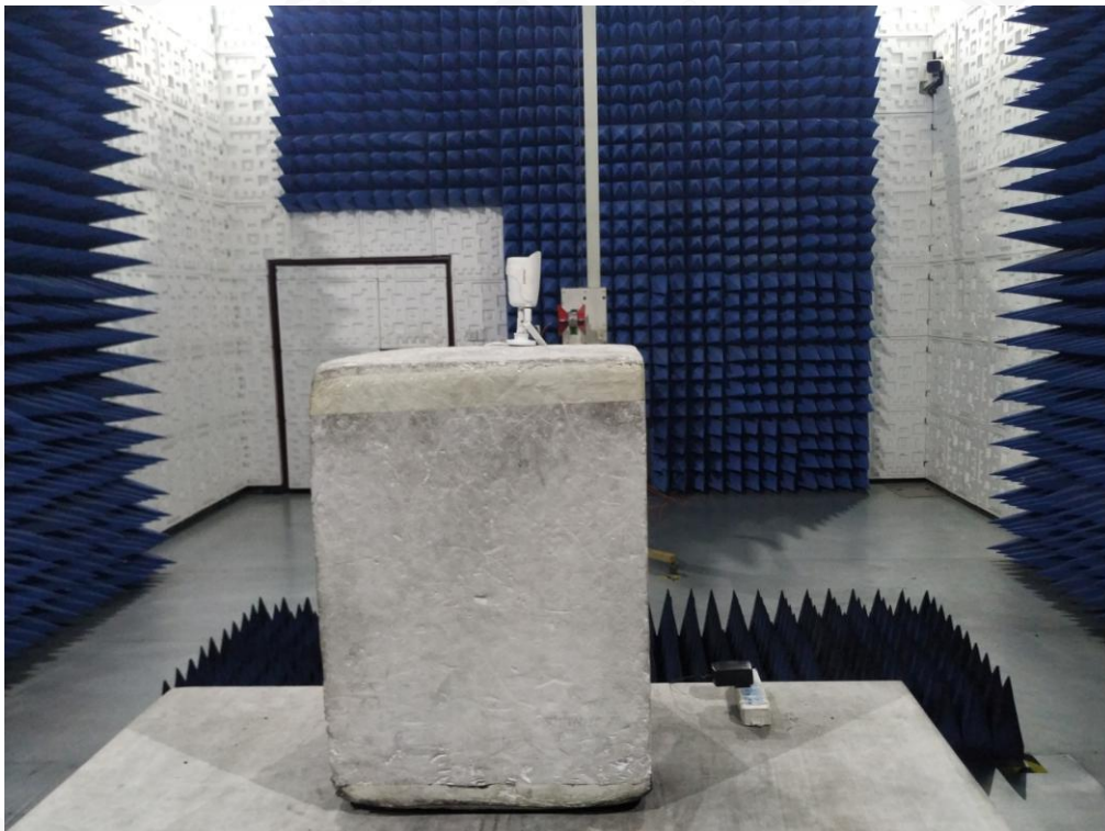
FCC RADIATED EMISSION TEST SETUP ABOVE 1GHZ
