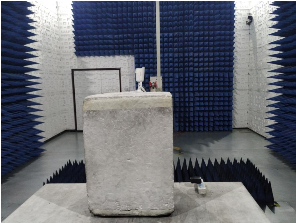
FCC RADIATED EMISSION TEST SETUP ABOVE 1GHZ
