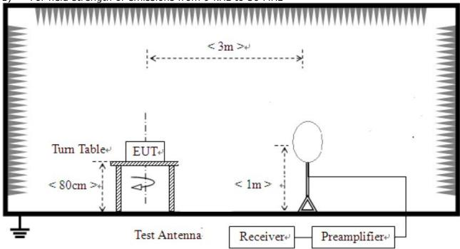
For field strength of emissions from 30 MHz to 1 GHz
