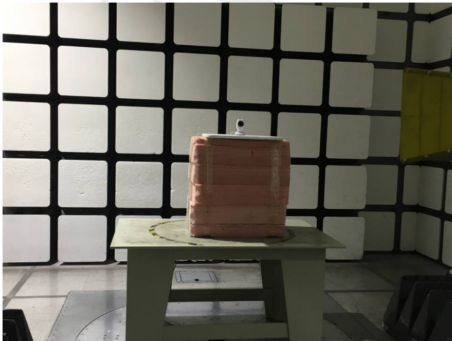
Radiated Emissions View (Above 1 GHz)
