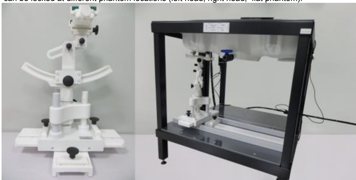
Device holder supplied by SATIMO
