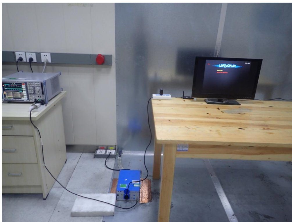
FCC RADIATED EMISSION TEST SETUP BELOW 1GHZ
