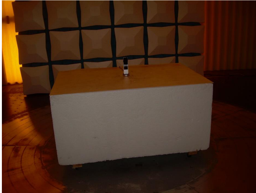
Photograph 1: Front View Radiated Emissions – In Charging Base – Below 1000 MHz
