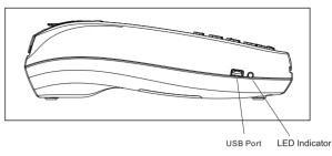
LED indicator: Power status indicator of device USB Port: USB communication interface
