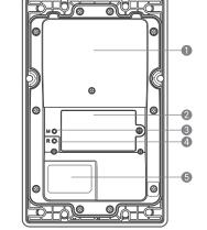
Port cover SIM/SAM card cover Menu for setup Reset Tag label
