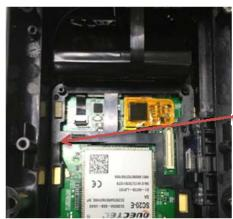
The cable line passes below the gap in the bracket.
