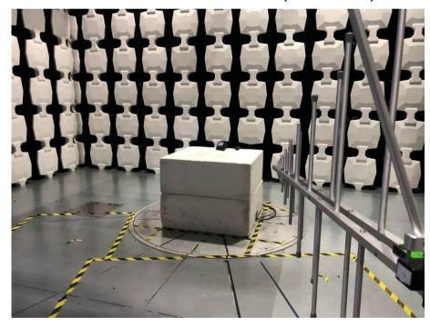
Picture2: Field Radiated Emissions (Above 30MHz)
