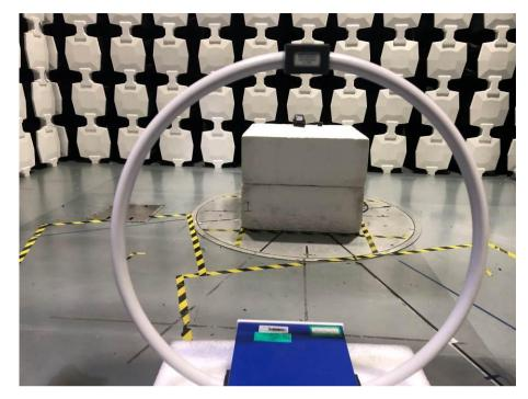
Picture1: Field Radiated Emissions (Below 30MHz)
