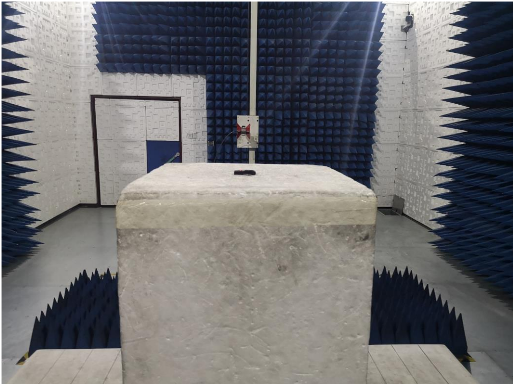
FCC RADIATED EMISSION TEST SETUP ABOVE 1GHZ
