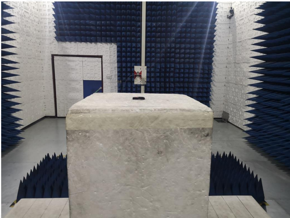
FCC RADIATED EMISSION TEST SETUP ABOVE 1GHZ
