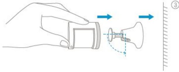
\*Suggest installation height is 1.2 2.1 m, less than 1.2 meters detection range has shrunk, but does not affect the use; Sensor will appear at the bottom of the blind area is greater than 2.1 m, parts can't detect.
